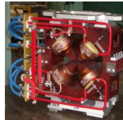
Quadrupole with GO steel
