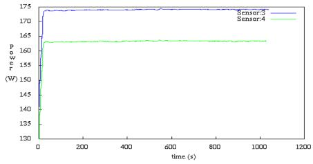
Both power readings show approx. 338 watts - basic power device verification
