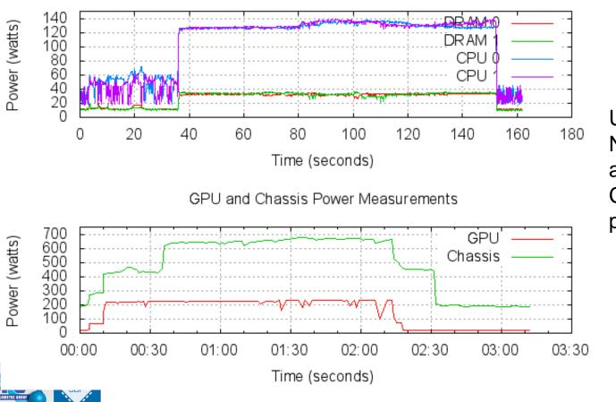
Use RAPL, IPMI and NVML, to give CPU and DRAM, Chassis and GPU power readings.
