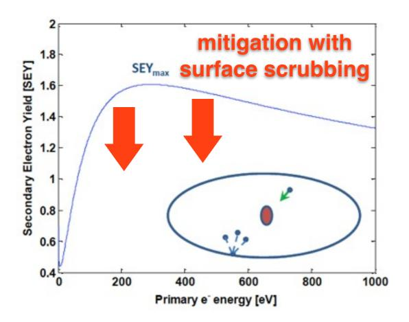
In 2011, 4 days of scrubbing at 50ns beams + 2 days of tests with 25ns beam 2012 : "EC free" operation
