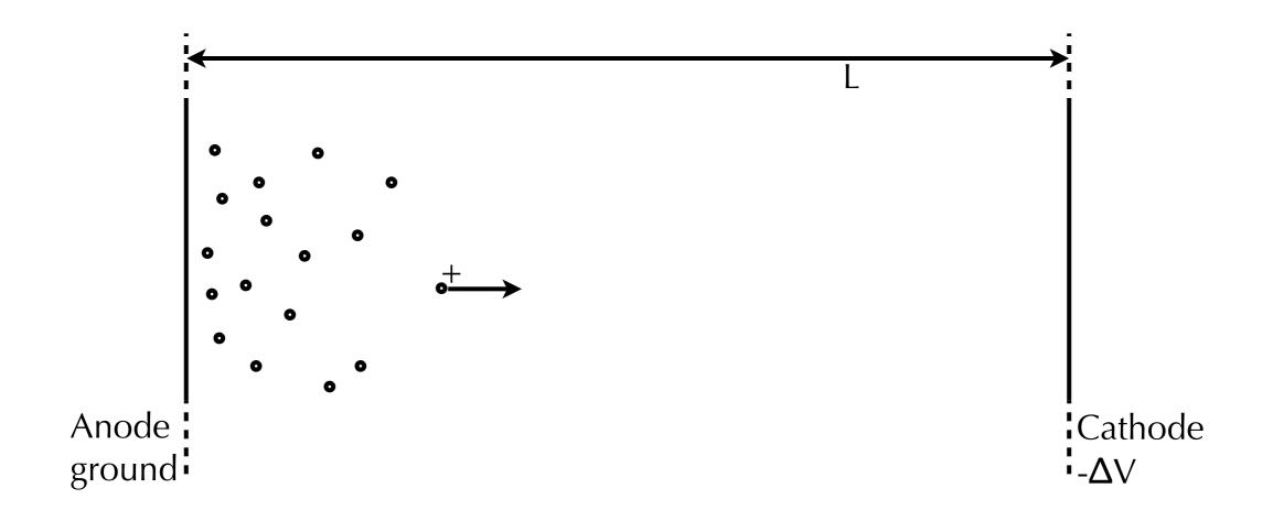
Infinite parallel plates at distance L with a potential difference of  $\Delta V$ At t = 0 uniform electric field of  $E_0 = \Delta V/L$ Positive ions generated at the anode at a constant and uniform flux R lons moving towards the cathode at speed v =  $\mu E$ Actual electric field E modified by the charge distribution
