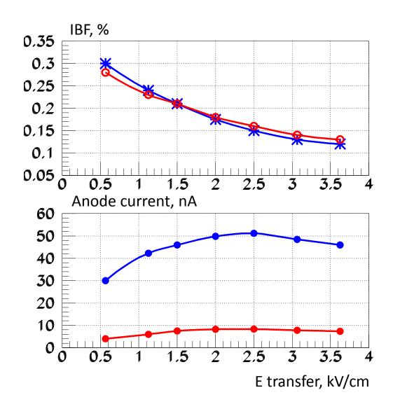
V mesh = 485 V Drift field = 0.4 kV/cm Induction Field = 0.125 kV/cm dV1 (GEM) = 195 V dV2 (GEM) = 225 V
