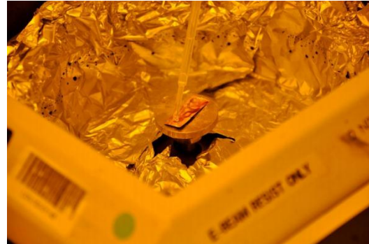
Small part of foil cut and spin-coated with PMMA
