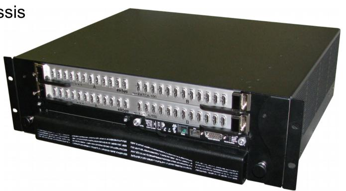
96 ADC channels = 12288 readout channels
