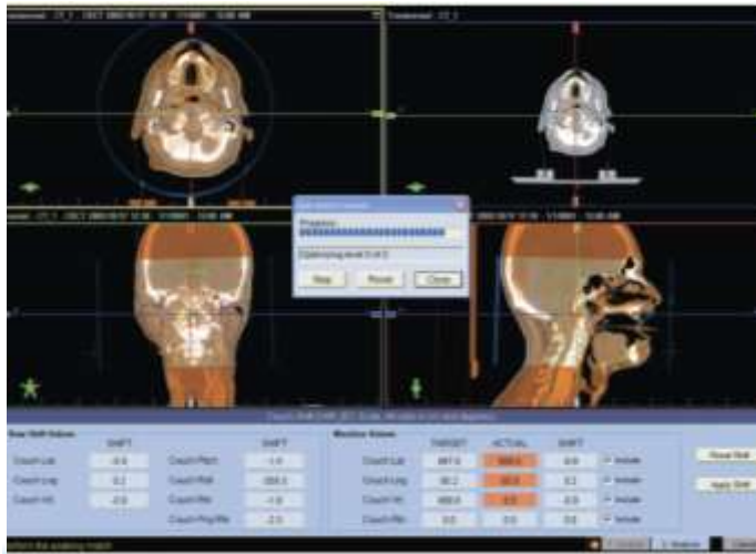
Figure 10. Volumetric registration at the treatment unit. A cone-beam CT acquired at the time of treatment is registered to the treatment planning CT (larger dataset) to properly position the patient on the treatment table (courtesy of Peter Monroe, PhD, Varian Medical Systems).
