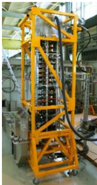
CERN LHC, TH 2167 klystron in lab and in UX45 cavern 16 klystrons delivering 330 kW @ 400 MHz, into operation since 2008
