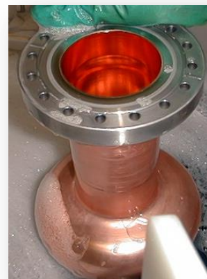
Copper test cavity (1300 MHz)
