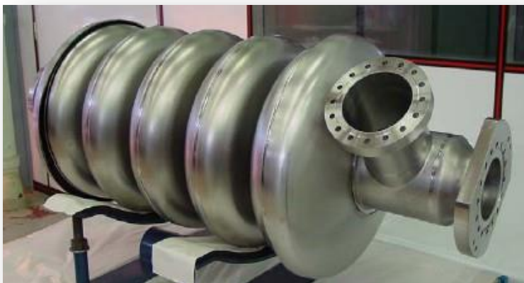
Superconducting cavity 5 cells Niobium for SPL (700 MHz)
