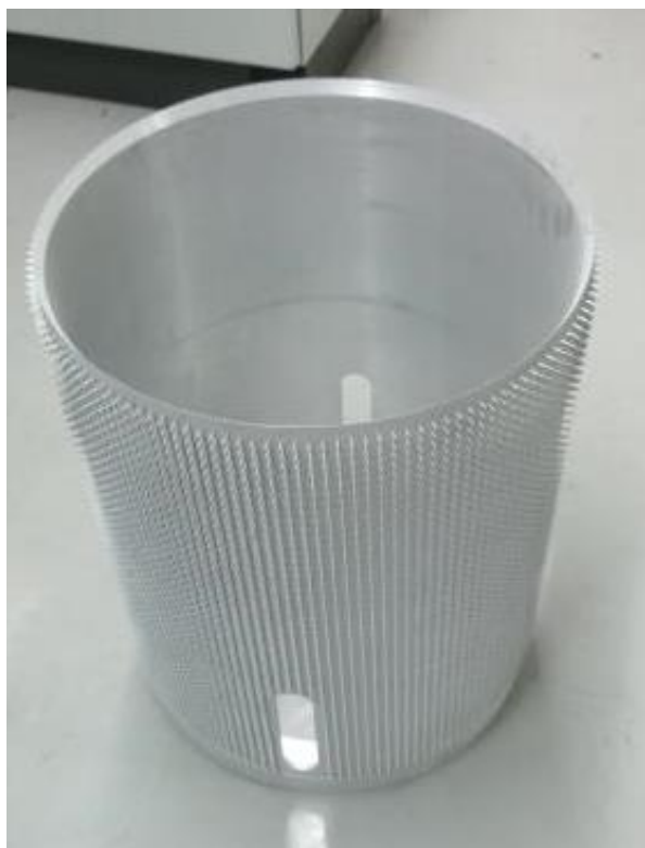
3500 pins on Carbon Cone flange for mechanical connection
