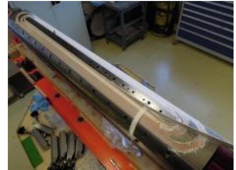
QXF coil wound in US [G.Ambrosio et al., ASC 2014]
