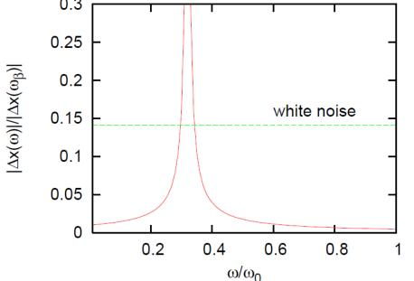
Beam response for sinusoidal and white noise
