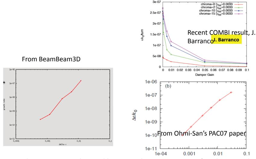
Good agreement is obtained between the BeamBeam3D simulation and Ohmi-San's PAC07 paper for the LHC parameters with 1 IP and 1 error.
