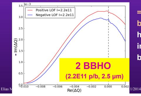
=> Previous limits can be increased by factor ~ 30 => Could therefore help to collide even earlier if impedance of Crab Cavities cannot be reduced sufficiently
