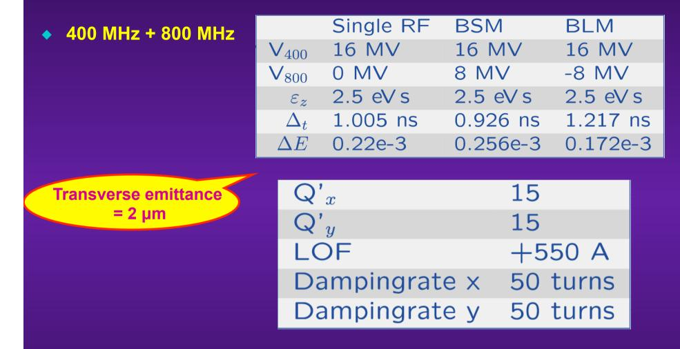
Studies made with the baseline impedance model (CFC collimators and no Crab Cavities): single-bunch sim. with HEADTAIL code
