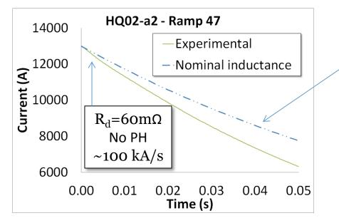
HQ simulation using the nominal inductance, experimentally measured at low dI/dt (<50 A/s)<sup>[1]</sup>
