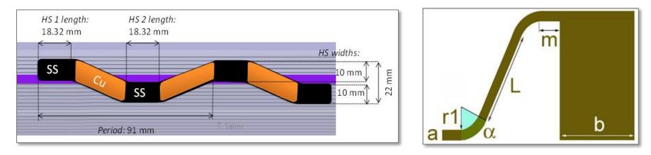
The protection heaters are designed in order to avoid as best as possible the damages coming from helium bubbles
