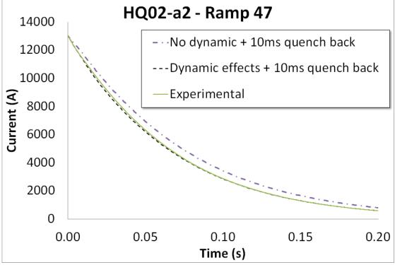
Quench back after 10 ms together with dynamic effects allow to reproduce the decay until its end
