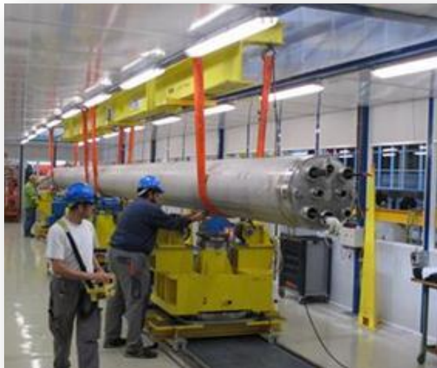
Cold mass transfer to the finishing bench
