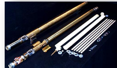
Existing QIMM and DIMM magnetic measurement rotating coil systems
