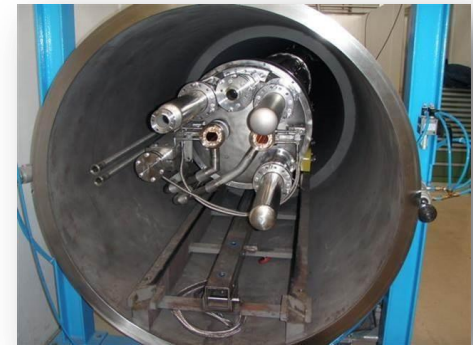
Insertion in the pressure/leak test tank
