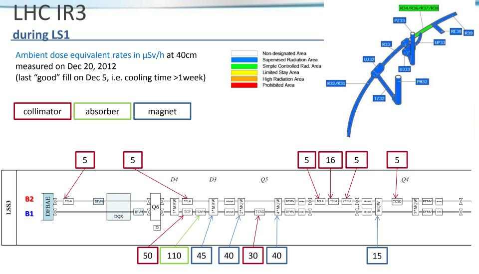
Ambient dose equivalent rates are 10-40 times lower than in IR7 (reflecting the sharing)
