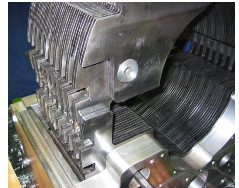
assembly of top and bottom yoke stacks for J-PARC SCFM
