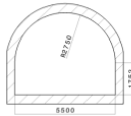
Crab Cavity Tunnel. Local enlargement
