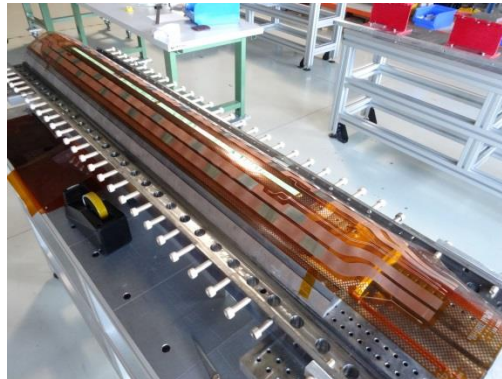
CERN coil #101 (Low-grade) Prep. for impregnation
