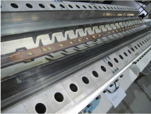
CERN coil #001 (Cu) completed
