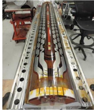
CERN coil #101 (Low-grade) Prep. for impregnation
