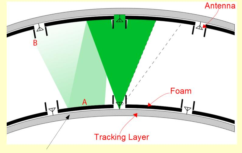
shielding by carbon-foam absorber
