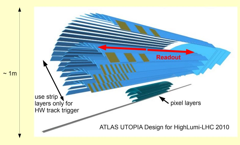
$\rightarrow$  additional cables (material) required for hardware track trigger
