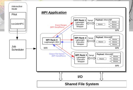
Schematic of the 'Yoda' extension of PanDA's Jedi dynamic job manager into HPCs as an MPI based service. Being implemented by the BNL, LBNL and UT Arlington based team that has implemented the event service and ported PanDA to HPC (ORNL Titan). The Yoda work's first target is NERSC HPCs.
