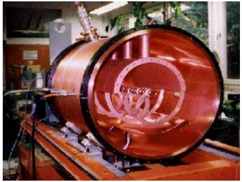
Fixed Structure! f = 101.28 MHz Zeff = 53 MΩ/m Q = 5400 - 5600 1,6 MV @ 90 kW
