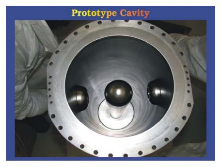
E<sub>acc</sub>T= 6MV/m over a length of 18 cm = 1.08 MV @ 7W power dissipation on LHe.
