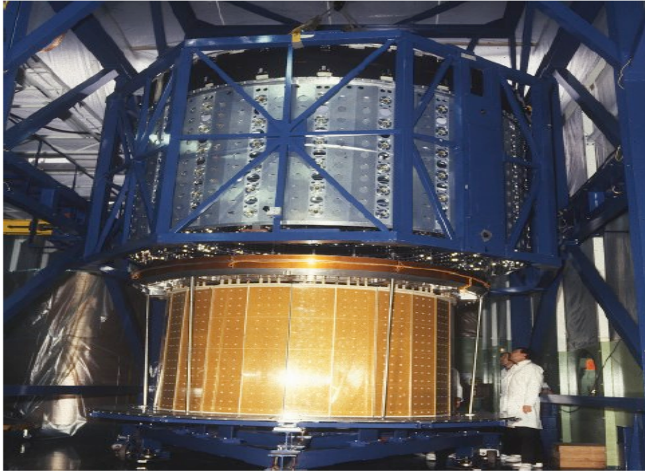
Fig. 20: DELPHI RICH detector being inserted into the mirror's barrel.
