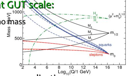
Run parameters to low scale with renormalisation group equations to calculate masses at 1 TeV scale
