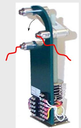
The moving part of the mechanical relay is bouncing sometimes (loss of contact)
