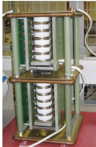
New Crowbar Switch (Thyristor stack)
