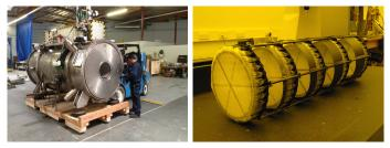
Each plane is a layer of scintillating fibres, rotated 120  $^\circ$  to their neighbours.
