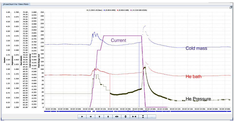
Heater never operates; less excess cooling power than FC1
