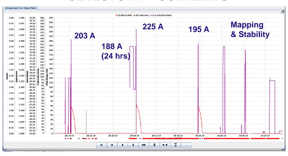
Two true quenches; one – 225 A – caused by hard limit in psu
