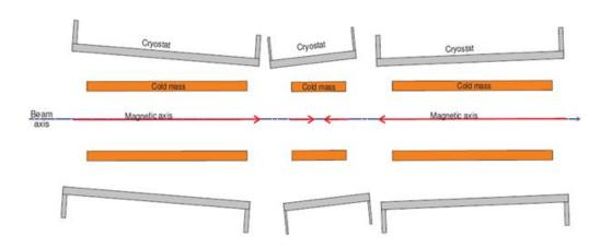
Need to know position of *magnetic axis* to 0.25 – 0.5 mm to align axes of modules to beam axis
