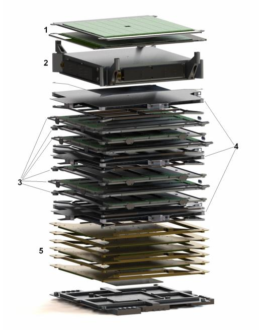
The NUCLEON apparatus includes the charge measurement system consisting of the 4 pad silicon detectors layers (1), the energy measurement system consisting of the carbon target (2) and the silicon microstrip detectors divided by thin tungsten layers (3), the trigger system consisting of the 6 scintillator layers (4)
