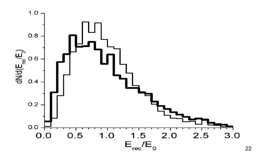
Calorimeter reconstructed energy distributions for 100, 150 and 200 GeV electron beams (solid line) in comparison with simulation results (dashed line) and Gaussian fits for experiment (thin solid line) and simulation (dotted line). RMS~8%
