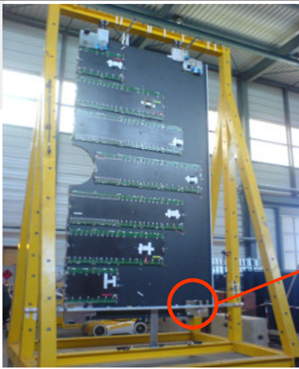
Deformations spaceframe and TPC insertion test
