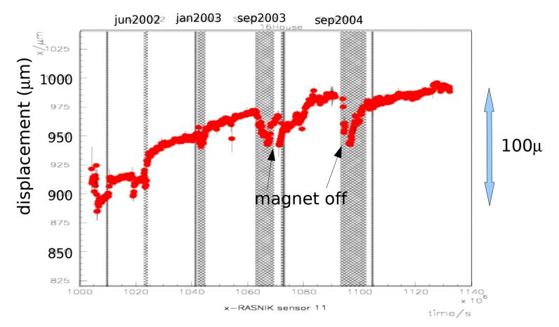
$\bullet$  Periodically correct the global alignment of the Si to keep misalignment w.r.t COT within  ${\sim}20\mu m.$
