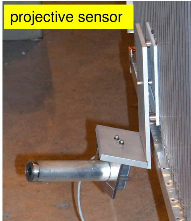
reference plate mounted on toroid
