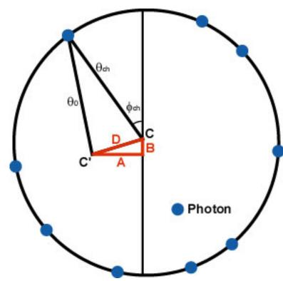
$$\Delta \vartheta = A\cos(\varphi_{ch}) + B\sin(\varphi_{ch})$$
