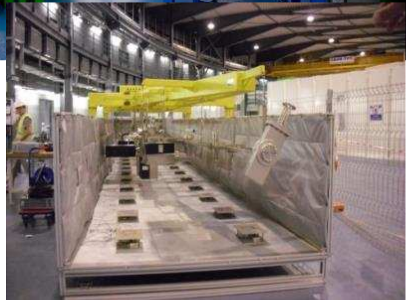
Bake out oven (length 14m,height 1m,width 2m)
