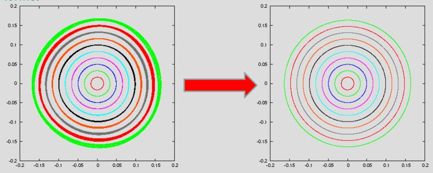
LHC at collision energy with strong Landau damping Octupoles switched on. Horizontal motion from  $1 - 10 \sigma$ .
