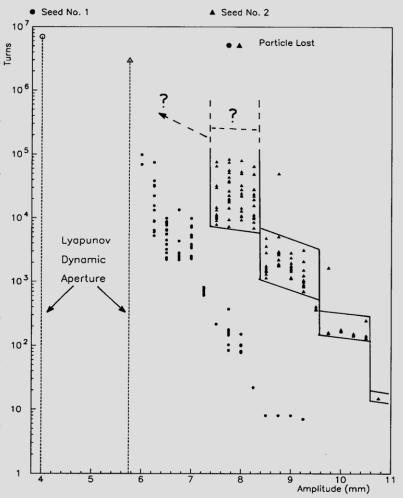
The survival plots depict the number of turns particles stay in the machine for a given amplitude. In this particular example we tracked an ensemble of particles started in a tiny volume of phase space. The width of the survival times tends to grow inverse proportionally with amplitude since the chaotic motion becomes weaker. There is no known method that could predict the evolution to smaller amplitudes toward the onset of global chaos.
