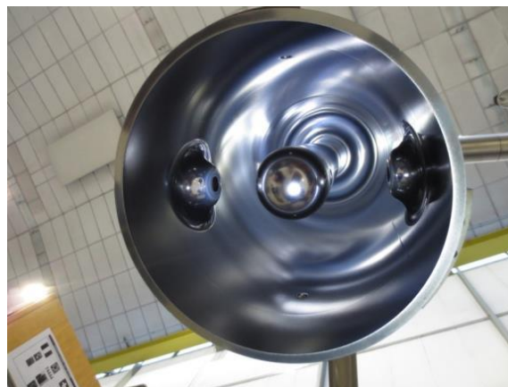
RF cavity coated with Niobium
