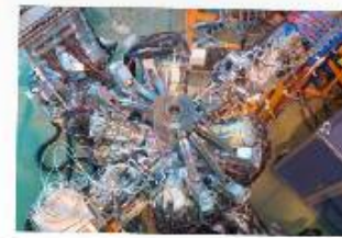
The MINIBALL gamma-ray spectrometer at the ISOLDE facility at CERN (as seen from above), where UWC researchers will carry out their measurements.
