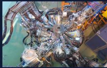
The MINIBALL gamma-ray spectrometer at the ISOLDE facility at CERN as seen from above, where UWC will carry out their measurements.
