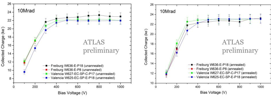
Also 10Mrad Gamma irradiation show no clear degradation on the collected charge
