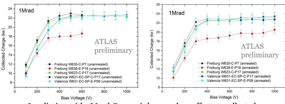
Irradiation with 1Mrad Gamma's has no clear effect on collected charge for most sensors
