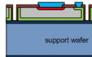
h) Contact holes, Al deposition and patterning
