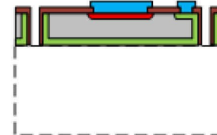
i) Removal of the support wafer
