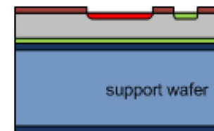
d) Oxide growth, lithography, etching and ion implantation to form doped regions
