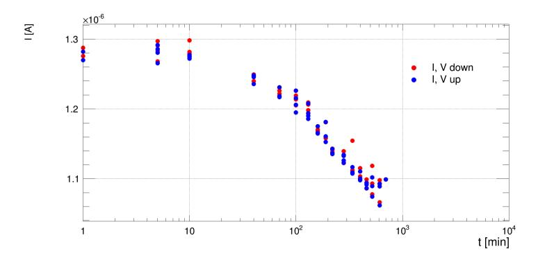
Corresponding values for current related damage rate are around 2·10<sup>-17</sup> A/cm, 1/3 of expected value
