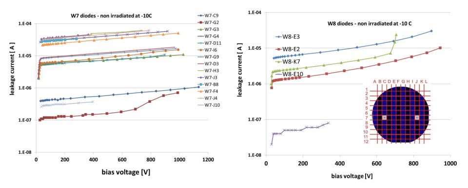
Devices have current spread in the range of 2-3 orders of magnitude and show no apparent gain variation over the wafer.
