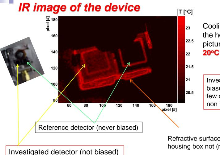
Cooling surface to which the housing (see left picture) is mounted is at 20°C measured with Pt-100
