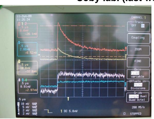
Red plot: Delta signal Blue plot: Sigma signal
