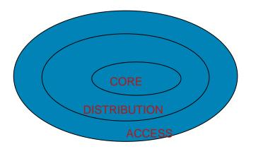
The Hierarchical Network Design Model Separates the Network into Three Functions
