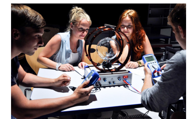
A fine beam tube, one of the many experiments featured in S'Cool LAB.
