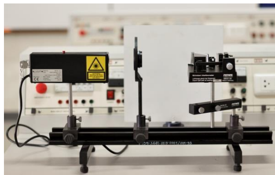
Figure 1 Instrument set up for measuring wavelength with Michelson interferometer
