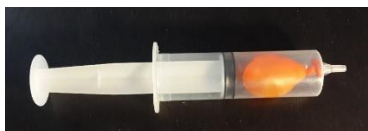
Figure 1 shown the experimental set for the demonstration of Boyle's Law
