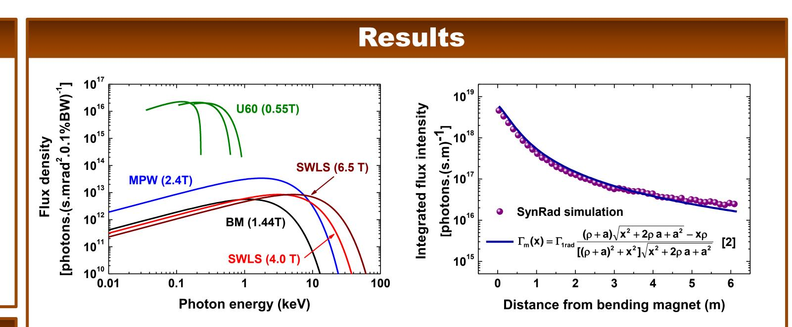
Left: SPECTRA [4] radiation spectrum of the bending magnet and insertion devices installed within the SPS storage ring at the beam current of 150 mA. Right: Integrated flux intensity (radiated from a bending magnet) along straight section from 3D SynRad simulation [5] and from calculation using relation proposed in [2].
