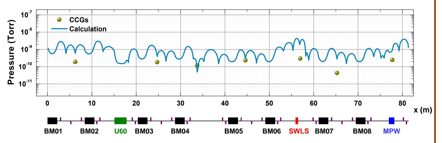
Calculated pressure distribution along the SPS storage ring at the averaged beam current of 115 mA and the photon dose of 2,000 A.hr, in comparison with measured pressure from CCGs. 3D simulations using SynRad and MolFlow are currently in progress.
