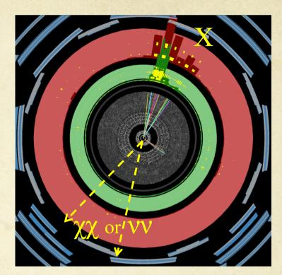
Display of a high  $p_T$  jets recoiling against missing transverse energy  $E_T$ (miss).
