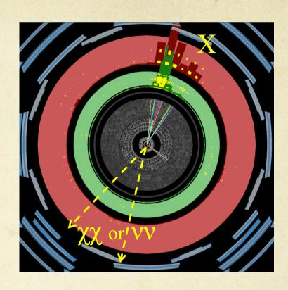
Display of a high  $p_T$  jets recoiling against missing transverse energy  $E_T$ (miss).
