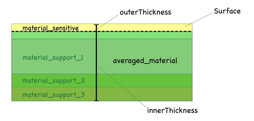
averaged material is automatically computed from detailed simulation model
