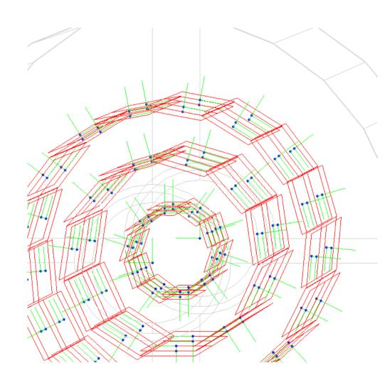
example: surfaces attached to ILD vertex detector in new DD4hep model ILD ported from Mokka
