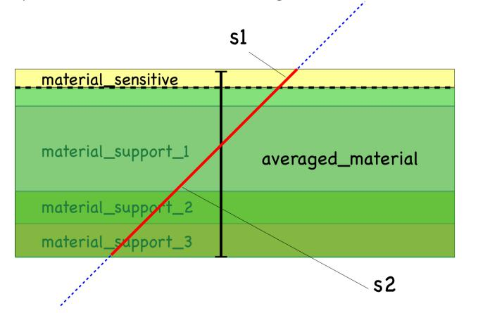
use material properties A, Z, rho, radLen, intLen to compute effect of energy loss and multiple scattering along path lengths "through the surface" s1,s2
